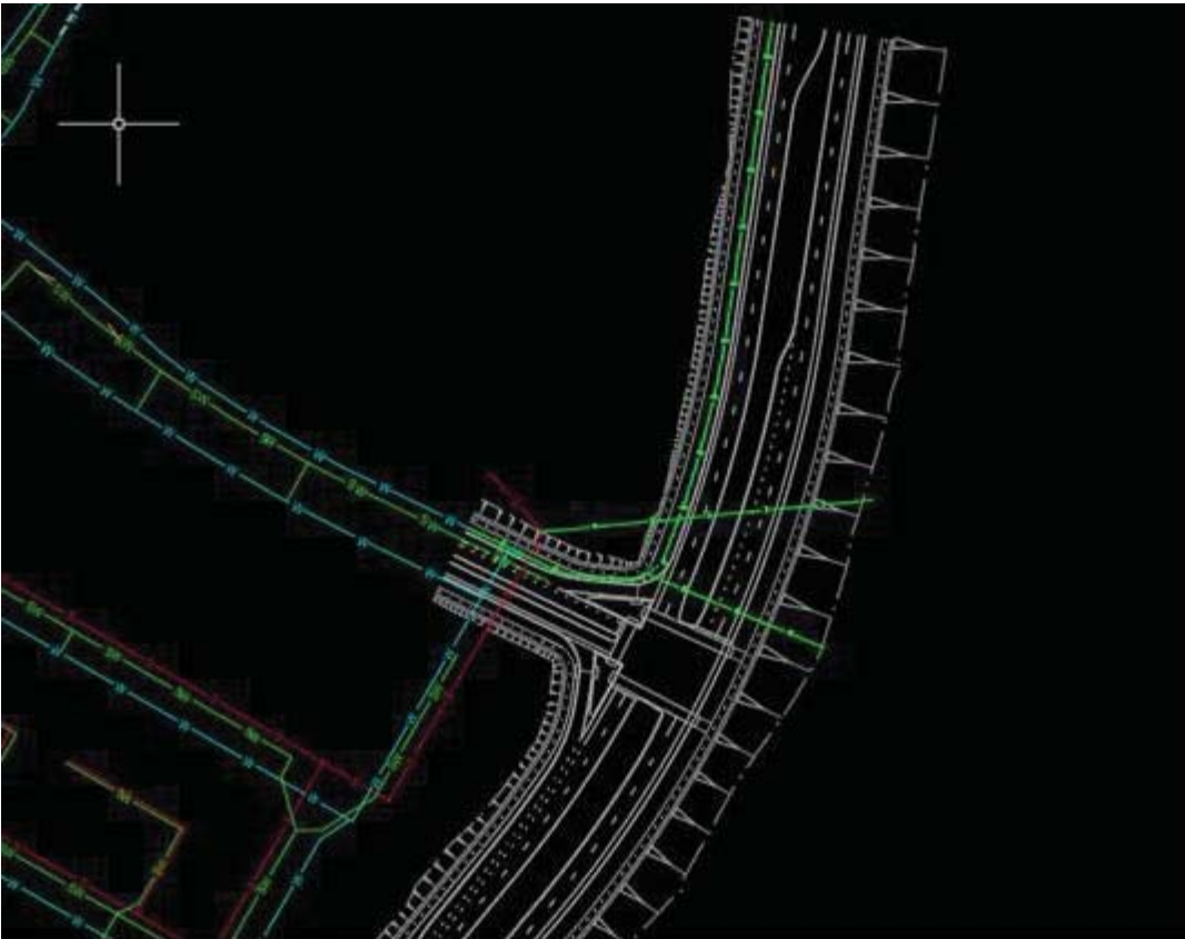
Figure 11.5: Tie in to Whitlam Estate utilities
