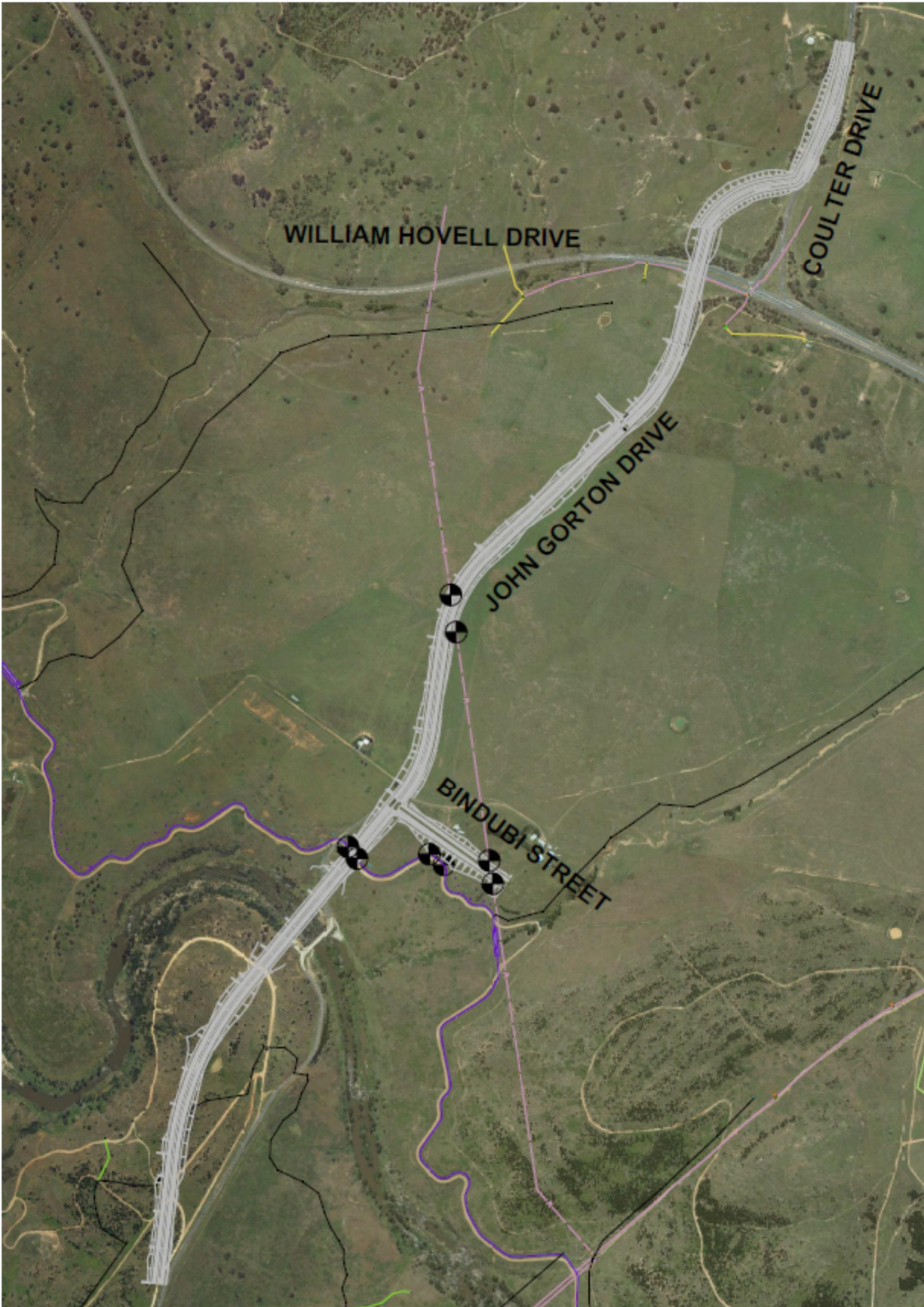
Figure 7 Pothole locations on Bulk Supply Water Main and MVIS
